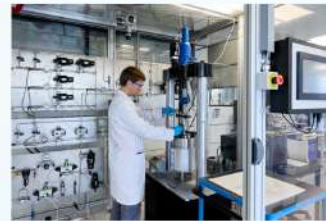
Fig 3. Rising load machine for testing in 100%H 2 and H 2 +CH 4 blends, in Tecnalia's H 2 TestLab facility
